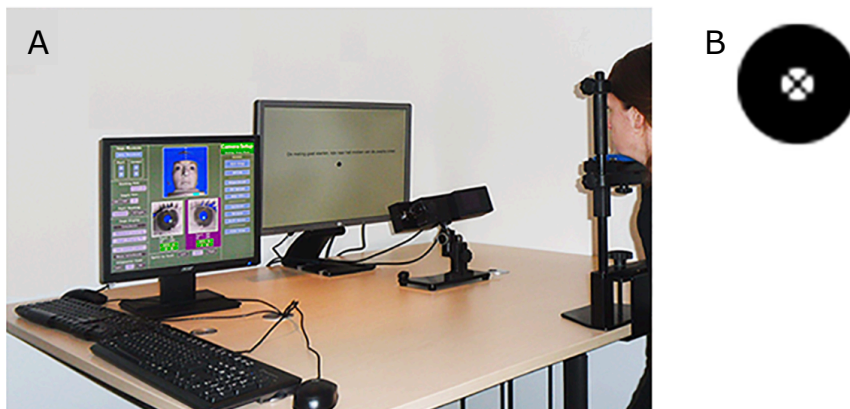
Figure 5: The set-up of the infrared oculography measurement (75)
